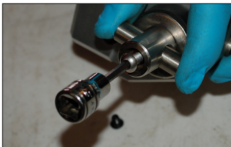
Loctite screw #2, tighten to small end of shaft
