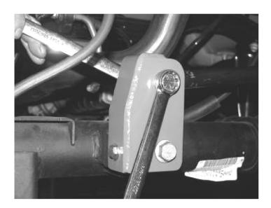
15. After marking the holes, remove the bracket from the axle and drill the 2 3/8" holes.
