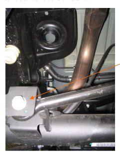
7. Place the new rear track bar bracket on the rear axle. Using the track bar bolt, bolt down the bracket and make a mark (using a punch or marker) where you will need to drill the two (2) new mounting holes.
