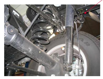
13. Remove the rear track bar at the axle end.
