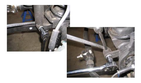
3. Disconnect the ABS line from the bracket on the steering knuckle on the driver side then the passenger side. Remove the factory shocks.
