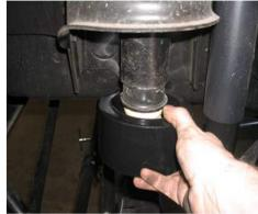
6. Pry out the factory bump stops and install the supplied bump stop extenders in the factory cups. Then install the factory bump stops in the lower end of the extenders. It may be necessary to lubricate the bump stops to fully seat them in the extenders.
