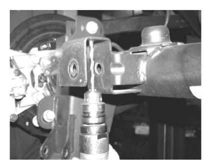
5. With the coil spring removed, install the Black Mountain lift spacer over the stock spring isolator.
