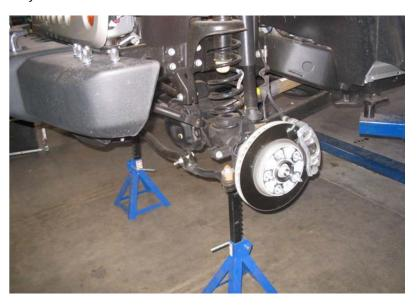
2. With the jack under the front axle, jack up the axle to remove the driver side and the passenger side wheels, disconnect the sway bar end link on the driver side as well as the passenger side.
