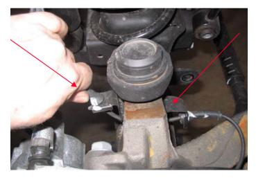
4. With the shocks removed, and sway bar and ABS line disconnected, lower the axle down to remove the coil springs on the driver side first, then the passenger side.
