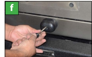
Remove stock tire carrier pad and replace screw
