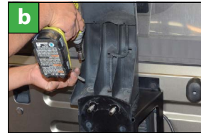
Unbolt brake light from stock tire carrier mount
