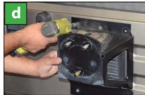
Unbolt stock tire carrier from tailgate
