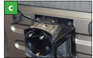
Gently pull wiring out of tailgate and tire carrier
