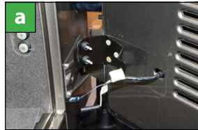
Disconnect wiring on inside panel of tailgate
