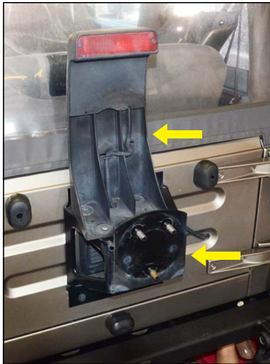
Disconnect wiring on inside panel of tailgate
