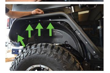
3. Install the supplied plastic spacers in-between the flare and the body of the Jeep on the rear four (4) bolt sleeves (see bottom photo) - then insert bolt through flare and spacer into fender hole of Jeep.
